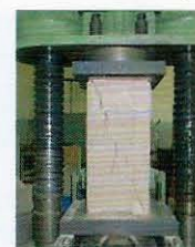
Figure 4. Testing bonded prism.
