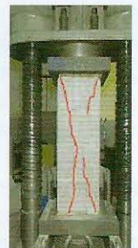
Figure 11. Four-unit prism bonded with mortar
