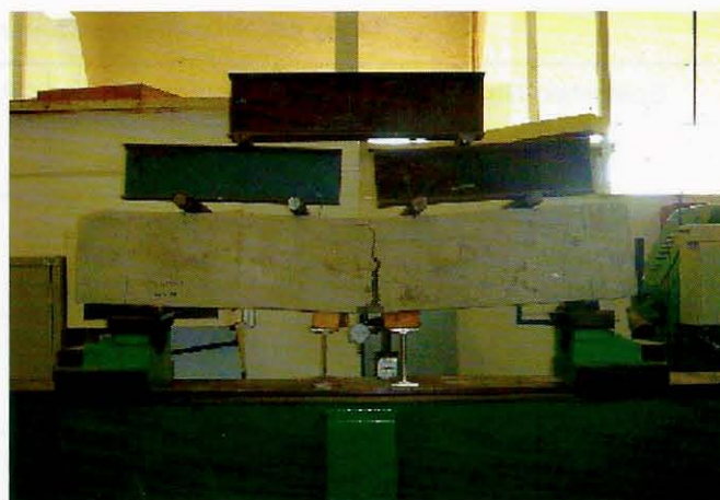
Figure 6: Load arrangement and mode of failure.
