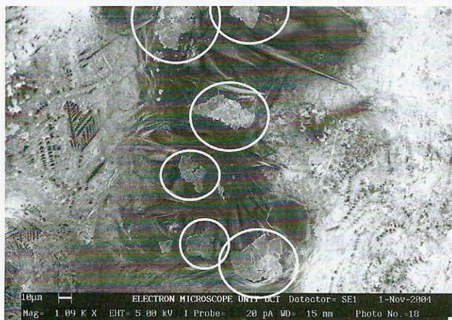
Figure 1: Secondary electron image of Friedel's Salt formation in an OPC mortar
