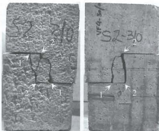
Fig. 5—Typical failure mode for plain C30/00 (both sides of same specimen).
