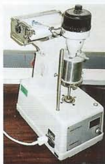
Fig. 5 – Variable speed viscometer (Visco-Corder)
