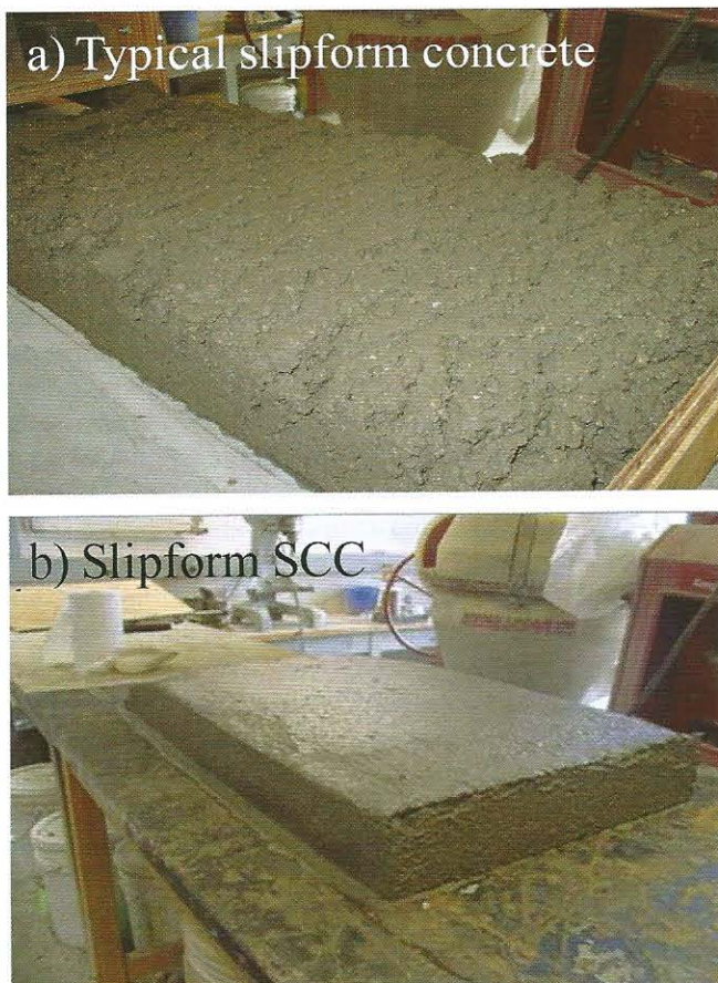
Figure 7. (a) Minipaver slab with typical slipform concrete. Rough surfaces indicate poor consolidation. (b) Minipaver slab with SF-SCC mix. Smooth surface indicates proper consolidation while straight edges indicate adequate green strength.
