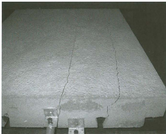
Figure 9. Longitudinal splitting cracks in specimen A.
