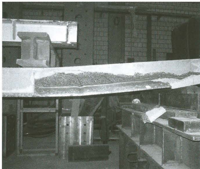
Figure 7. Specimen A at the ultimate limit state.
