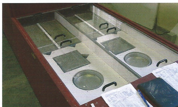
Figure 1: The test compartment of the climate chamber and mould used for crack measurements
