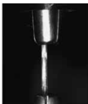
Figure 8: Test setup for creep of synthetic macro fibre (Babafemi & Boshoff, 2015)
