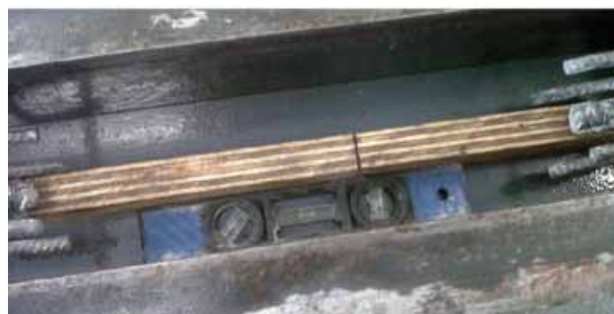
Figure 3: Alignment of hooks using spirit level
