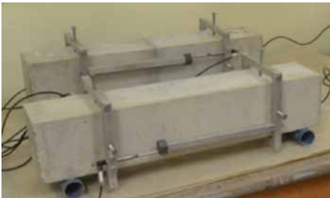
Figure 6: Drying shrinkage test specimens
