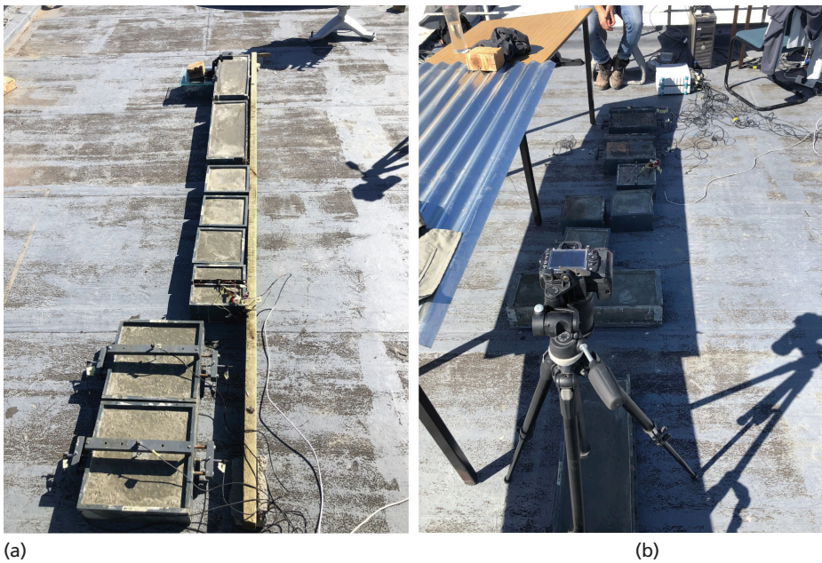
Figure 3: Test setup of (a) specimens in the sun; (b) specimens in the shade.
