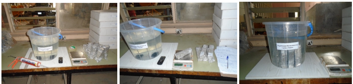
Figure 4: Samples Sealed with Impermeable Membrane, Weighed and placed in Water.
